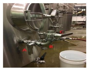
ii) Open valve C and add dosing solution to the elbow, then close valve C. {Figure E
